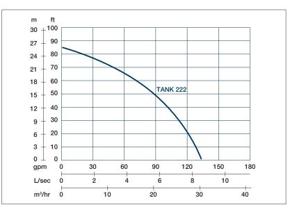
Shaft Speed : 2850rpmSolid Passage: 9mmOutlet : 50mm, 2inOUTPUTHEADFLOW2.2 kWRated : 15m, 49ftRated : 5 l/s, 79gpm3 HPMax : 26m, 85ftMax : 8.3 l/s, 132gpm
